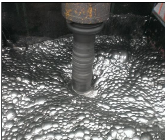
Figure 1. Flotation cell concentrating flake graphite
